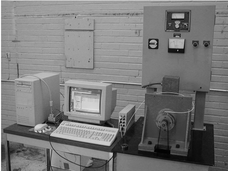
Fig. 4. Bearing test system and data acquisition set-up.
